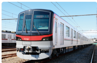
Lightweight aluminum alloy body
