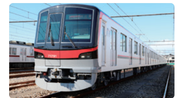
Lightweight aluminum alloy body
