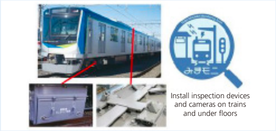
Facility monitoring systems (illustration)
